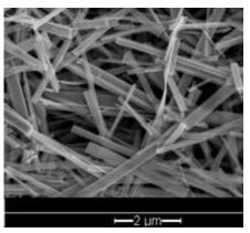
Analyzer that was developed using nano–structured  $K_2W_7O_{22}$  (pictured to right) and with research support from a Sanford NDSU Research Seed Grant.
